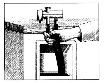
Press down on the thumb release. Lift the connector up onto the faucet and release your thumb pressure so the connector is held firmly in place.
